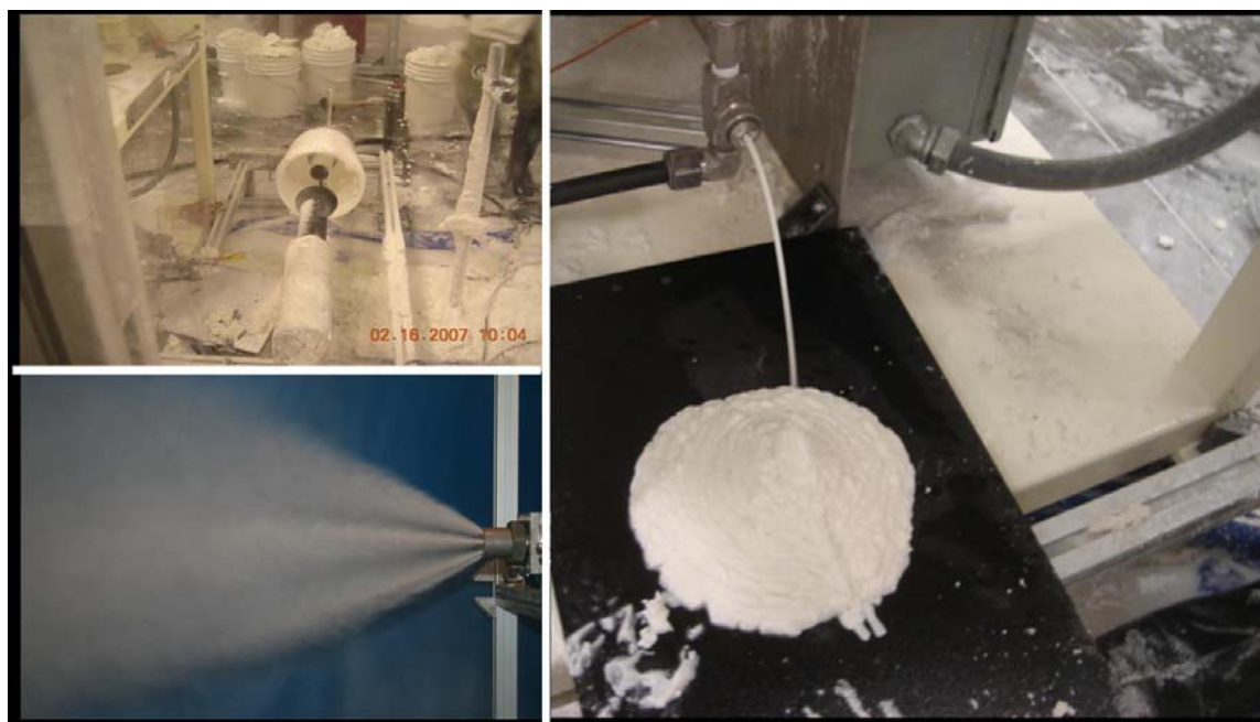
Figure 3. Some examples of spray drying atomization experiments at Procter & Gamble. Upper left: a view of our lab during detergent slurry atomization trials. The Oxford laser spray visualization system is shown. Lower left: pneumatic atomization of a proprietary feedstock. Right: detergent slurry flowing through a pneumatic nozzles with the air off. Note the consistency of the material.
